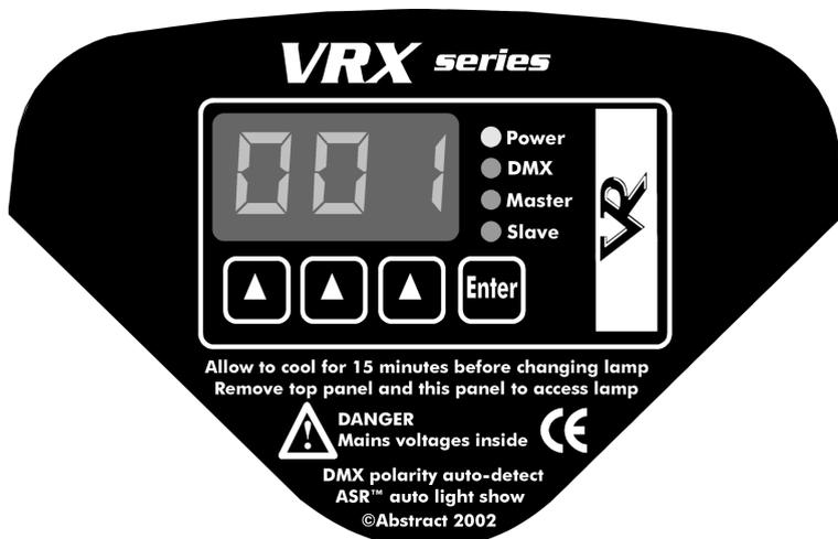
**Power light** (red). This light should be on whenever the unit is powered up. If it doesn't come on there is either no power to the unit, or some internal problem with the unit.
